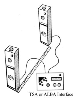
The switch on the top of your Sound Switch is the reset switch. The knob on the rear of the unit is for adjusting the sensitivity. Connect the DIN plug to either DIN socket at the rear of TSA/ALBA.
